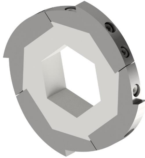
Fig. 4. 3D model of the cutting blade
