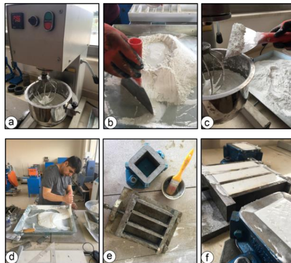
Fig. 2. Sample preparation: a) mixing calcite and white cement, b) adding water, c) adding chemicals, d) homogenous mixing of ingredients, e) preparation of molds, f) placing the mixture in the mold
