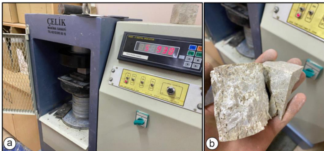
Fig. 4. Determination of compressive strength: a) test application b) broken sample
