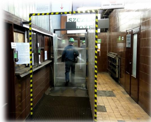
Fig. 8. A prototype of the UMID universal disinfecting installation in Budryk mine, made by Elektron s.c. [18]
