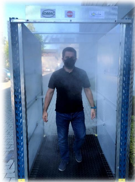
Fig. 12. Demonstration mist disinfection installation, when a person enters the main KOMAG building [21]
