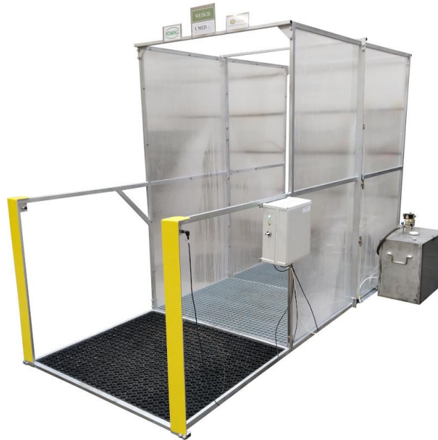
Fig. 10. Universal UMID mist disinfection installation - the serial solution used in coal mines [19]
