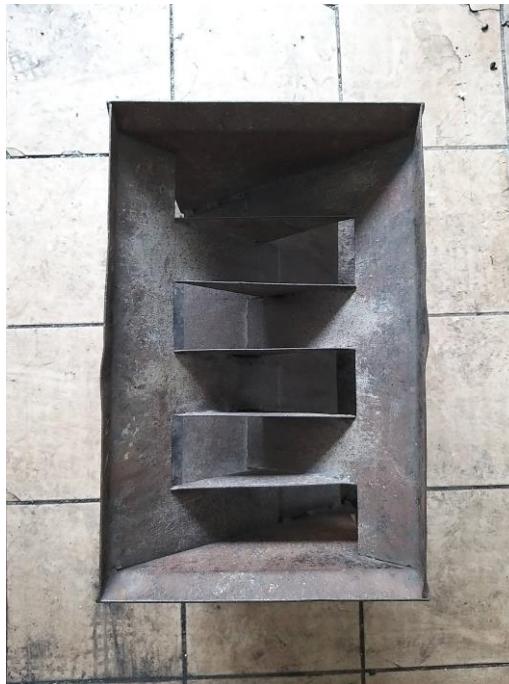
Fig. 7. Jones sample divider (own source)
