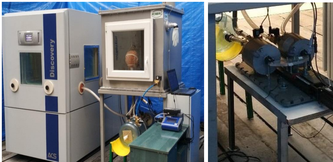
Fig. 3. Test stand for RPE equipment with a view of its artificial lungs on the right
