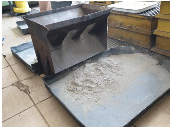
Fig. 2. Averaging the fly ash by the sample divider
