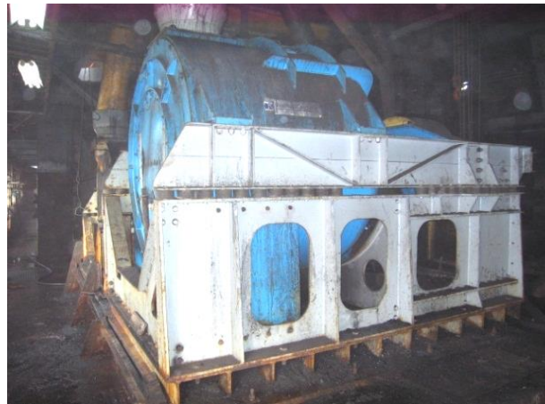
Fig. 3. WOK 1.5 centrifuge in sound-insulating enclosure [7]
