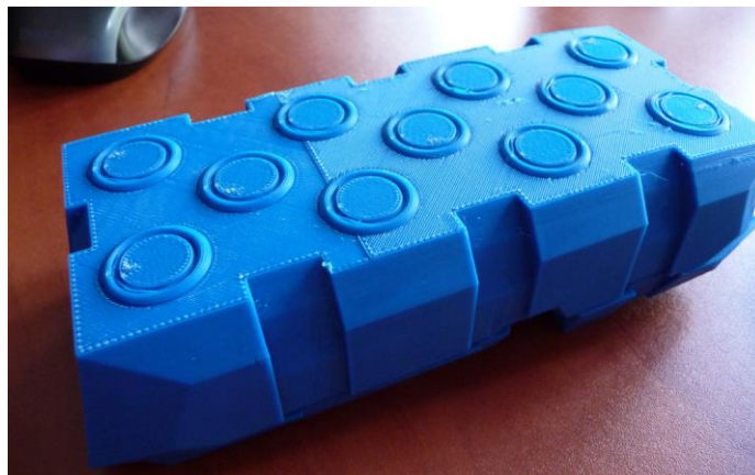
Fig. 1. Remote controller prototype – prototype including only external features of the device, with buttons mock-up - for testing the product comfort of use [5]
