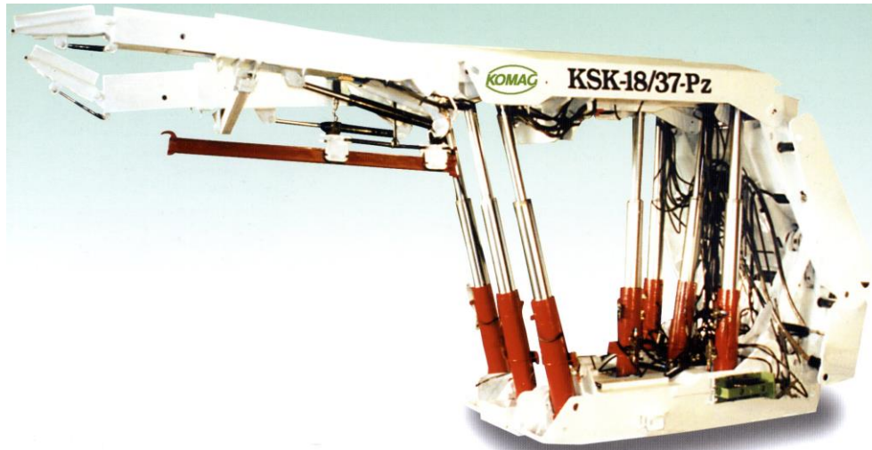
Fig. 4. KSK-18/37-Pz mechanized crossing unit [15]
